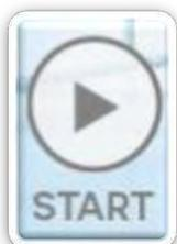
The START button is used to (re) start the tanning session and to program the parameters (please see Chapter 5). When the tanning time starts the colour of the section that indicates the time changes from white to yellow. During the cooling down time this section will turn red. In case a of a pause, the Start button can be pressed to continue the session. This has to happen before the pause time passes, otherwise the machine will proceed to the cooling down.
