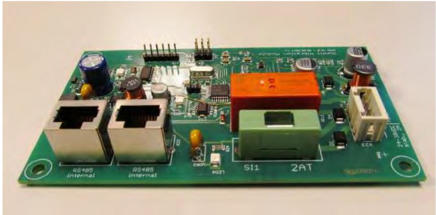
The VibraPlate module has its own 24 Volt connection, due to the power output that needs to be supplied to the motor of the VibraPlate.
